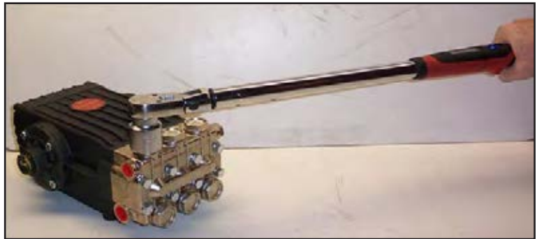
Figure 5-5. Replace Valve Cap and Torque to 95 ft. lbs.
