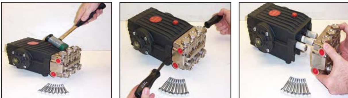
Figure 5-6. Separate Manifold from Crankcase
