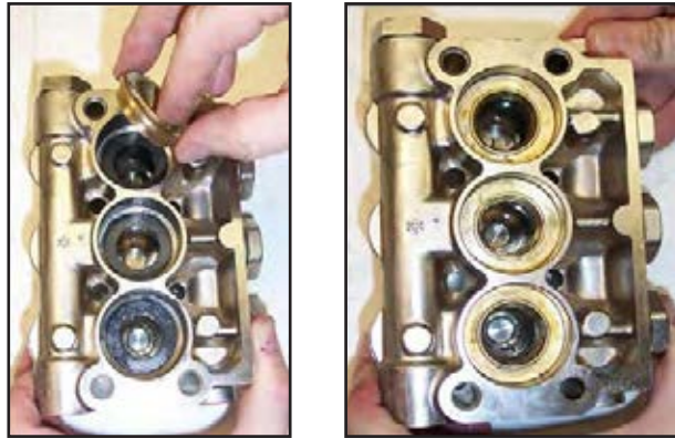
Figure 5-14. Install Retainers into Cavities
