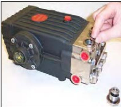
Figure 5-4. Apply Grease and Install Valves
