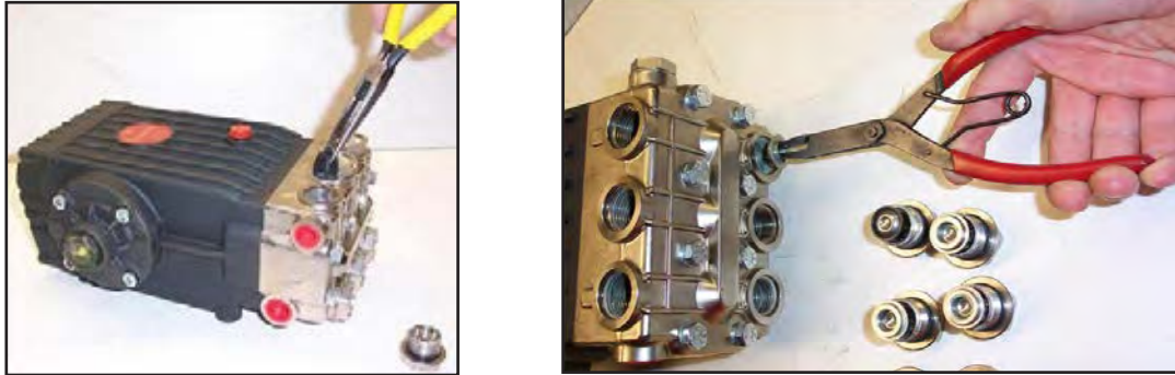
Figure 5-1. Remove Valve Cap and Valve Assembly
