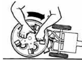
Figure 6-2. Loosen Cleaning Head Assembly
