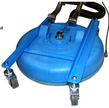
**Step 2:** Lift the handle off of the turbo deck. Place the concrete bracket on the of the turbo deck. Make sure the holes align.
