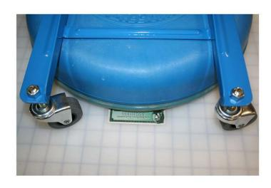
**Step 4:** Just the caster wheel so the boot ring or bursh ring is about the height of a credit card.
