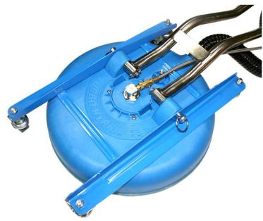
**Step 3:** Place cotter pin back in place. Securely connect the quick disconnect back on the swivel.
